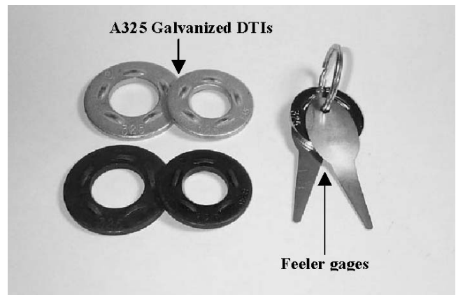
Figure 3-2. Direct Tension Indicators and Feeler Gages
