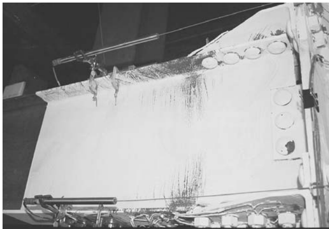
Figure 2-8 Web Local Yielding Limit State (SAC Project)
