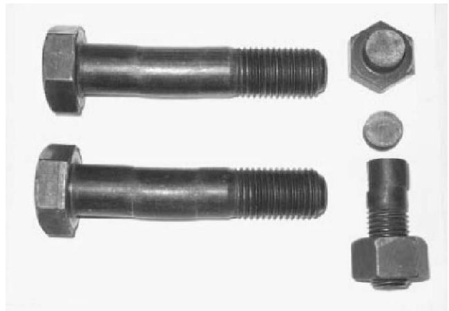
Figure 2-3. Bolt Shear Limit State (Photo by P.S. Green)
