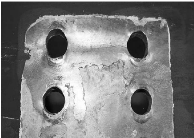
Figure 2-2. Bolt Bearing Limit State (Photo by J.A. Swanson and R. Leon, courtesy of Georgia Institute of Technology)
