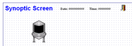
Finished tank object
