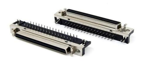
Starte right angle SCSI DB 68 female connector with latch bracket for PCB, this 90 degree HD 68 pin female SCSI connector pin arrangement in two rows, one on top of the other. The top row has 34 pins and the lower row has 34 pins. It is usually used on the Industrial equipment PCB and SCSI...
