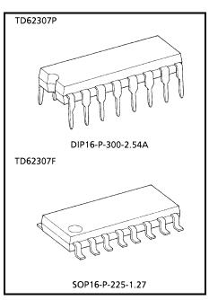
Weight DIP16-P-300-2.54A: 1.11 g (typ.) SOP16-P-225-1.27: 0.16 g (typ.)
