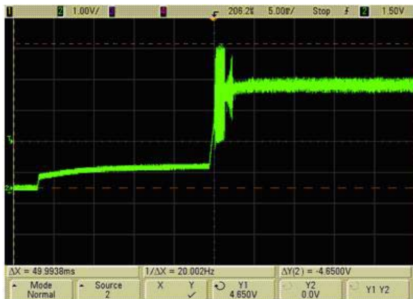
Figure 8. Input Voltage Overshoot >4V (Bad)
