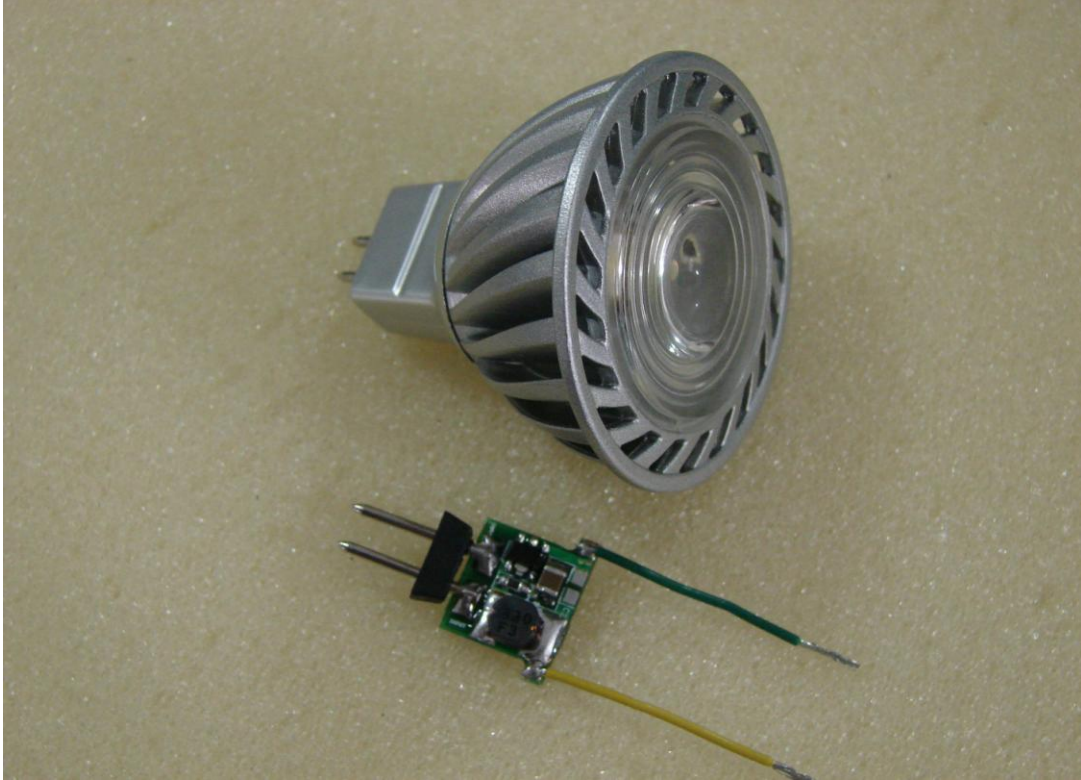
Fig 3 DEMO board for mass production
