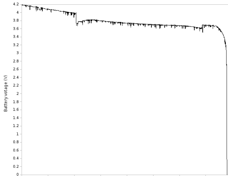
Figure 97: Typical discharging curve for battery
