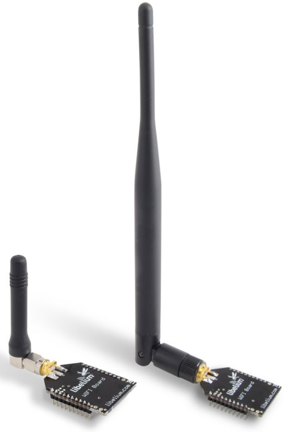
Figure 70: Wifi module with 2dBi and 5dBi antennas
