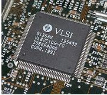
A VLSI VL82C106 Super I/O chip
