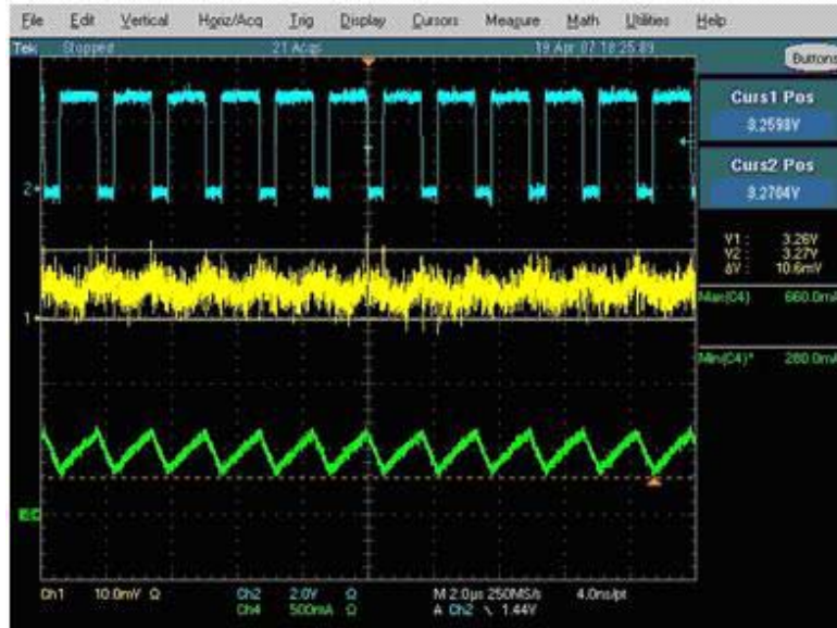
Figure 13. Ceramic 22 \mu F 1210 (X5R) (Good)
