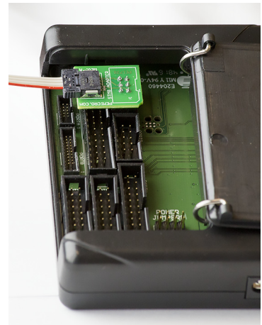
Figure 3-21: STM8 Adapter: 1) Bottom, 2) Top, 3) Connected To 6-Pin Header of Cyclone_Universal_FX (Adapter Sold Separately)
