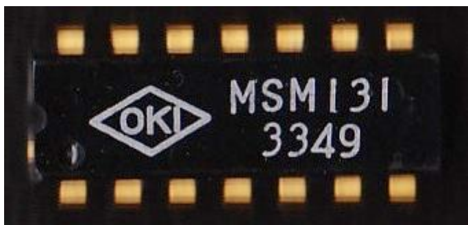
MSM131RS = Dual R-S Master-Slave Flip-Flop/1973
