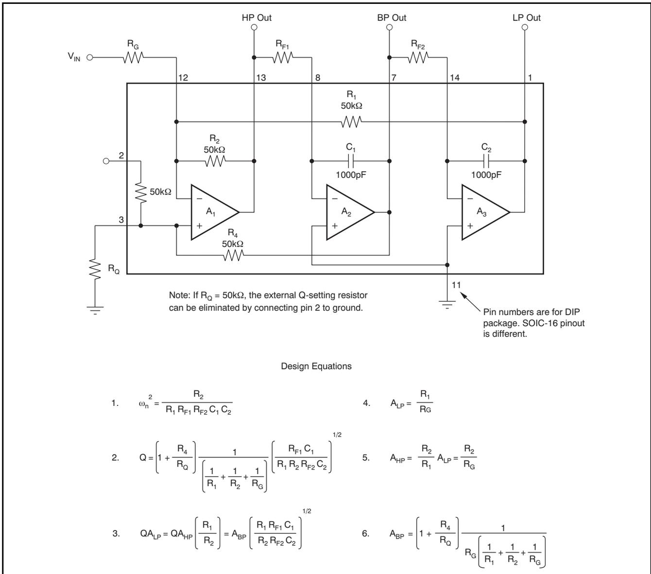
Figure 2. Inverting Pole-Pair
