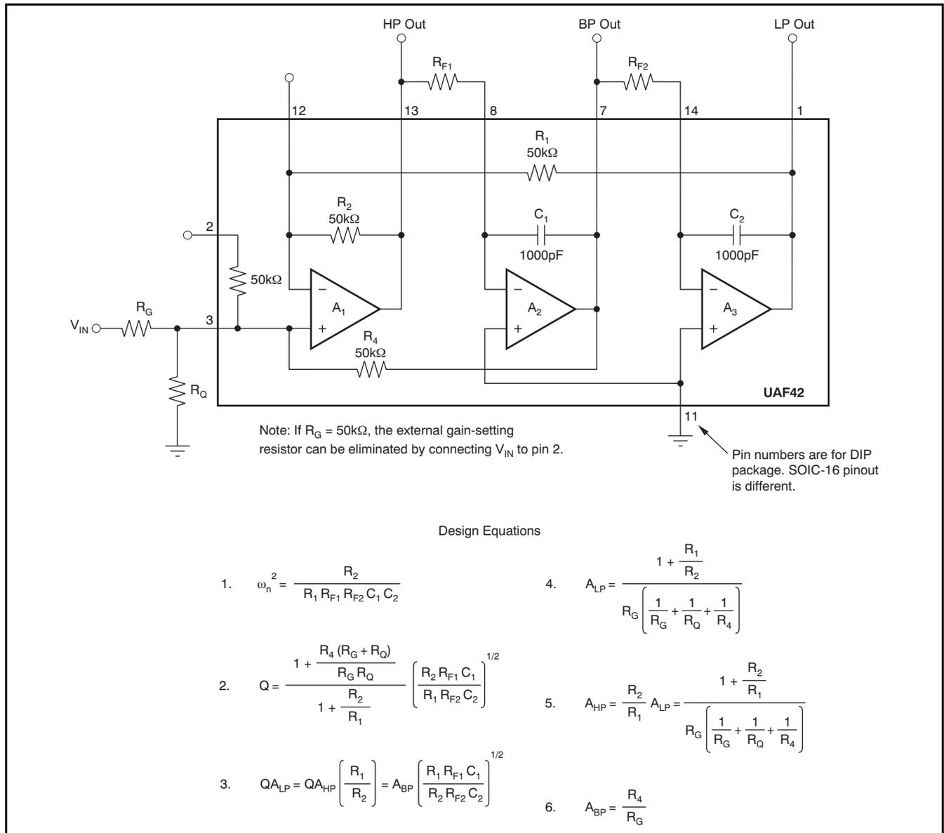
Figure 1. Noninverting Pole-Pair
