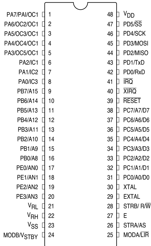
Figure 3 48-Pin DIP Pin Assignments
