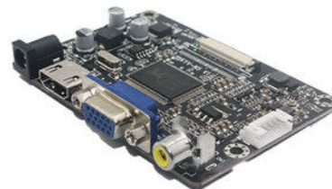
Standard HDMI/VGA Driver board for Customized Interface
