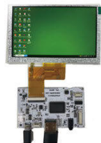
HDMI Driver board with micro USB power supply
