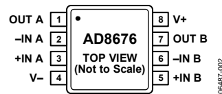
Figure 2. 8-Lead MSOP (RM-8)
