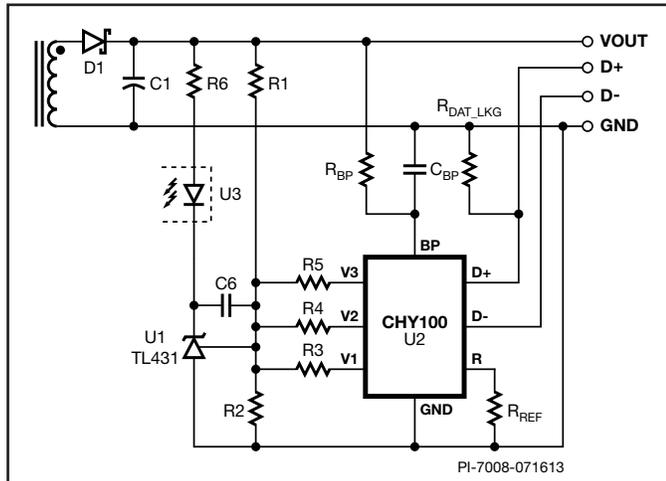
Figure 5. CHY100 with Traditional Output Regulation (CV Only).
