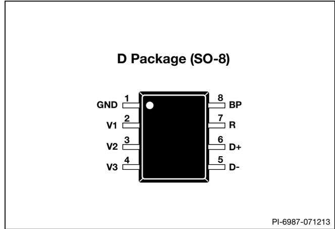
Figure 4. Pin Configuration.
