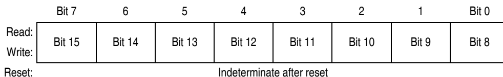
Figure 14-12. TIM Channel x Register High (TCHxH)
