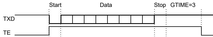
Figure 34-16. Example of TE Drive with Guard Time
