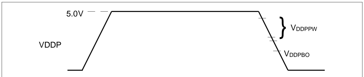
Figure 13 Supply Threshold Parameters
