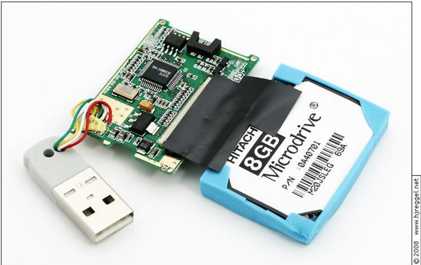
USB Plug, PCB and Microdrive with Shock Protection
