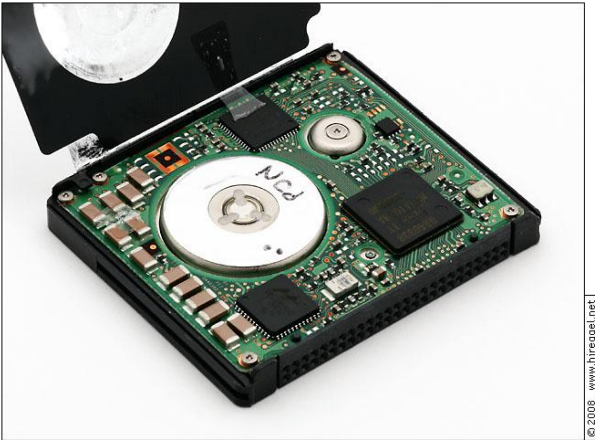
Hitachi 6GB Microdrive HMS360606, Main PCB
