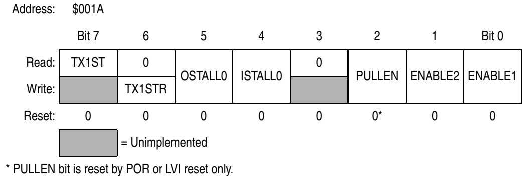
Figure 9-22. USB Control Register 3 (UCR3)
