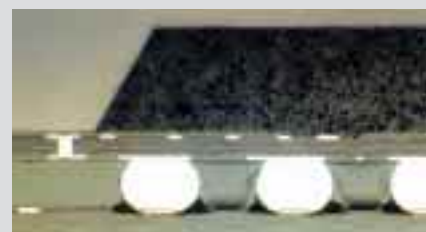
Cross-section of PBGA after soldering
