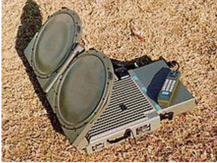
JGSDF JPRC-C1 SATCOM (Satellite Communications) terminal
