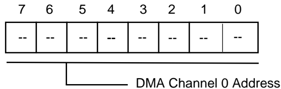
Figure 55. DMA Source Address Register 0L
