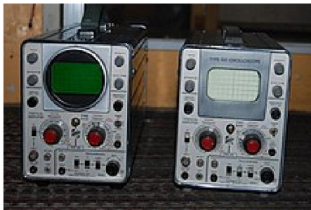
Tektronix 321- Their First Battery Operated Transistor Oscilloscope. LEFT- Later Version RIGHT- Earliest Version
