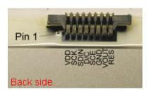
Dont forget a 470nF capacitor beetween Vout and GND!
