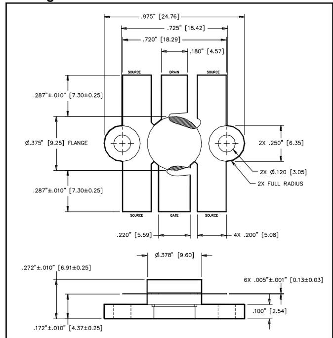
UNLESS OTHERWISE NOTED, TOLERANCES ARE INCHES  $\pm .005$ " [MILLIMETERS  $\pm 0.13\text{mm}$ ]
