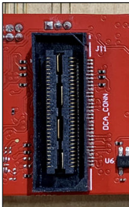
Figure 2-15. DCA1000 HD Connector (J11)
