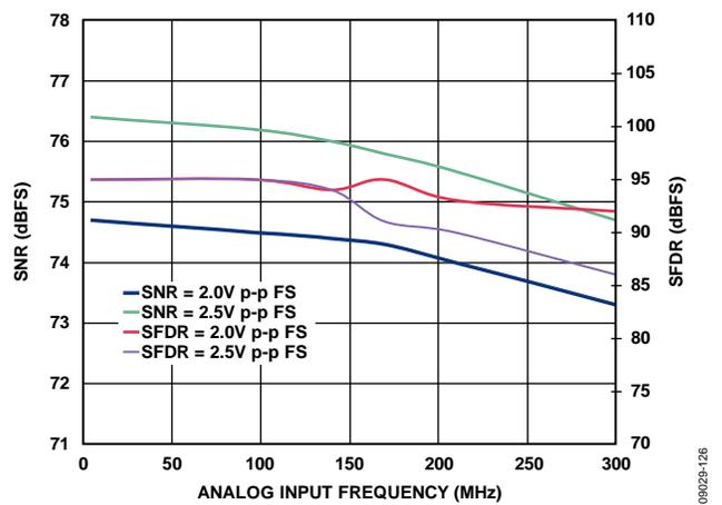
Figure 26. SNR/SFDR vs.  $f_{IN}$ , 2.0/2.5 V p-p FS, AD9467-200
