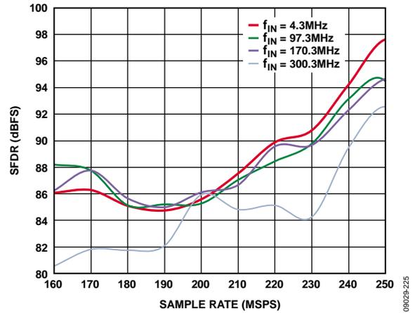
Figure 25. SFDR vs.  $f_{SAMPLE}$ , 2.5 V p-p FS, AD9467-250
