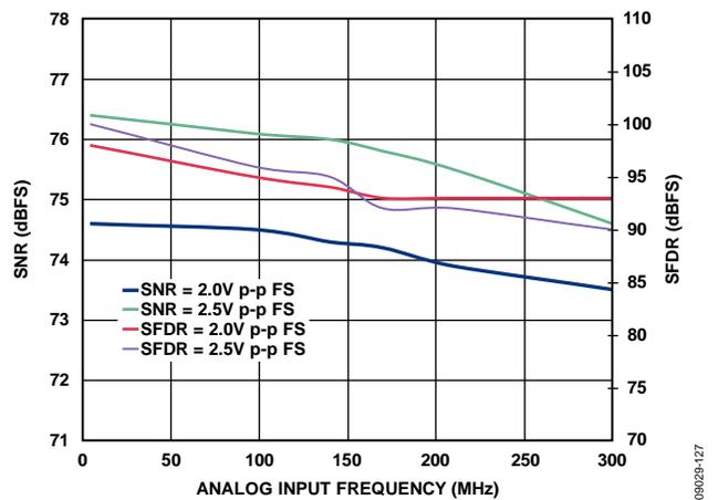
Figure 27. SNR/SFDR vs.  $f_{IN}$ , 2.0/2.5 V p-p FS, AD9467-250
