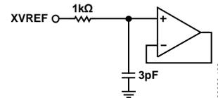
Figure 9. Equivalent External VREF Input Circuit (When Enabled)
