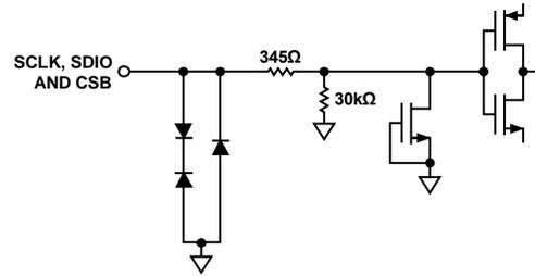
Figure 7. Equivalent SCLK, SDIO, and CSB Input Circuit
