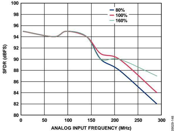
Figure 50. Buffer Current Sweeps, 2.5 V p-p, AD9467-200
