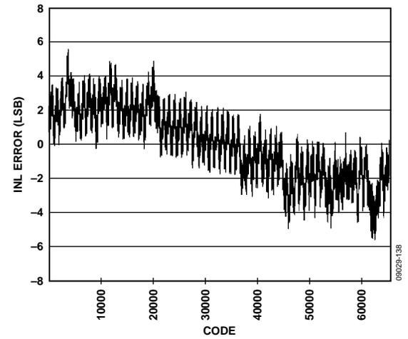
Figure 38. INL,  $f_{IN} = 4.3$  MHz, 2.5 V p-p FS, AD9467-250
