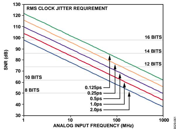
Figure 61. Ideal SNR vs. Input Frequency and Jitter
