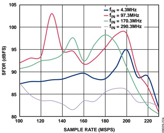
Figure 24. SFDR vs.  $f_{SAMPLE}$ , 2.5 V p-p FS, AD9467-200
