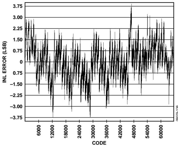
Figure 36. INL,  $f_{IN} = 4.3$  MHz, 2.5 V p-p FS, AD9467-200
