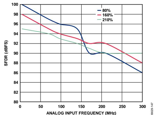
Figure 49. Buffer Current Sweeps, 2.5 V p-p, AD9467-250
