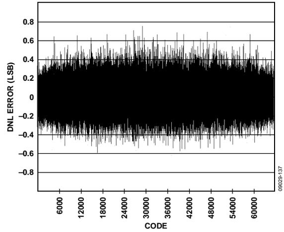
Figure 37. DNL,  $f_{IN} = 4.3$  MHz, 2.5 V p-p FS, AD9467-200
