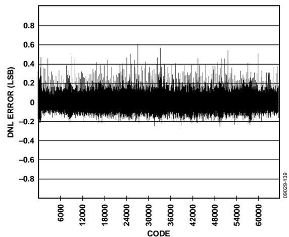
Figure 39. DNL,  $f_{IN} = 4.3$  MHz, 2.5 V p-p FS, AD9467-250
