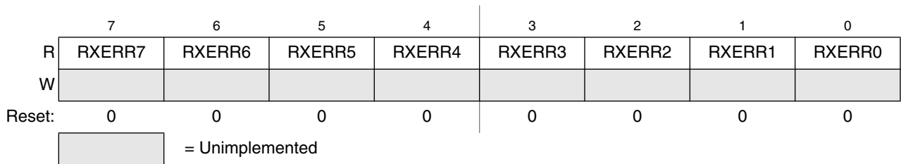
Figure 12-17. MSCAN Receive Error Counter (CANRXERR)
