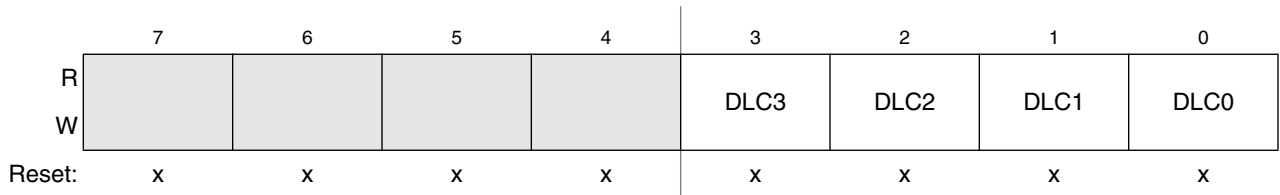
Figure 12-34. Data Length Register (DLR) — Extended Identifier Mapping
