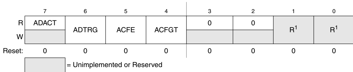
Figure 10-5. Status and Control Register 2 (ADCSC2)
