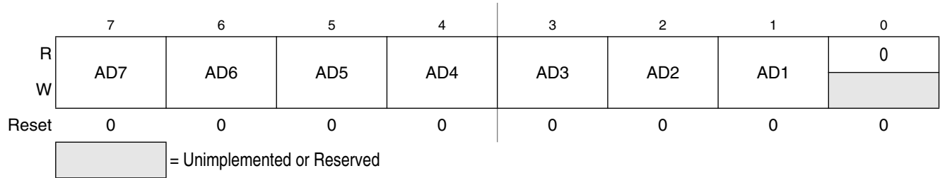
Figure 11-5. IIC Address Register (IICA)
